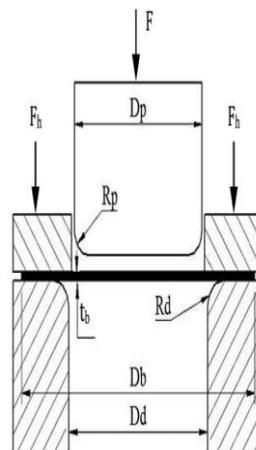
**Fig-4: SCHEME OF CUP DRAWING PROCESS**
