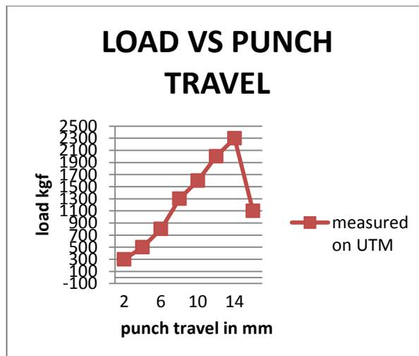
**FIG-13(B) COPPER LOAD VS PUNCH TRAVEL ON EXPERIMENT**
