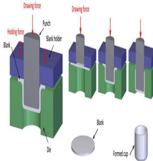
**Fig-3: SCHEMATIC ILLUSTRATION OF CUP DRAWING PROCESS**
