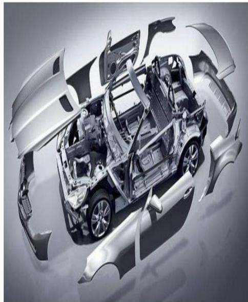
**Fig-2** AUTOMOTIVE PARTS PRODUCED BY SHEET METAL FORMING
