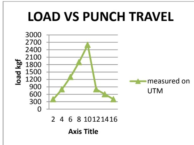
**FIG-13(C) BRASS LOAD VS PUNCH TRAVEL ON EXPERIMENT**
