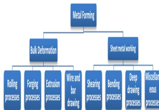
**Fig-1: CLASSIFICATION OF METAL FORMING PROCESSES**
