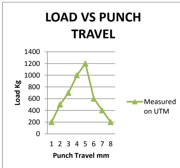
**FIG-13(A) AL 1100 LOAD VS PUNCH TRAVEL ON EXPERIMENT**
